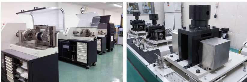
Thread Fastener Tightening Characteristic Testing Unit
